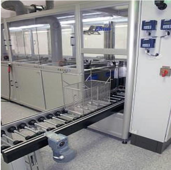
(As soon as its code has been read in, the batch passes through the Elma ultrasonic cleaning system.)
