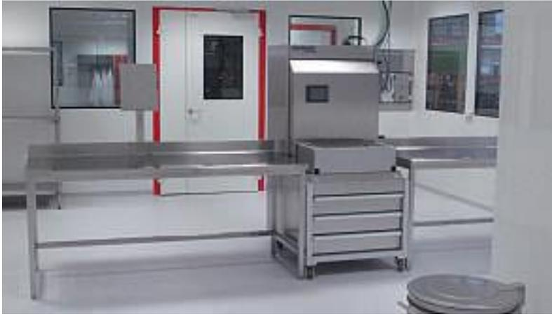
**Clean room ISO 7: in the centre of the packaging system with assembly table, material air locks at the rear, washing machine on the left, labels air lock on the right.)**
